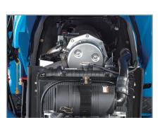
Shibaura ISM Tier 4 Engine 3 cyl, low vibration, fuel efficient yet powerful
