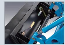
SKC bucket, front end loader with skid steer compatible bucket
